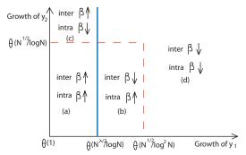
$y_i$ : expected total base inter-domain traffic sourced by a single node.  $y_s$ : expected total base intra-domain traffic sourced by a single node.
