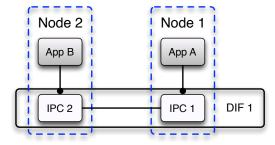
Third AppB allocates a connection to AppA using the communication service provided by the underlying DIF1. Once the connection is created, AppB keeps sending simple messages to AppA.
